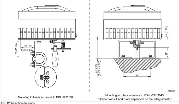
Fig. 12: Mounting drawings
