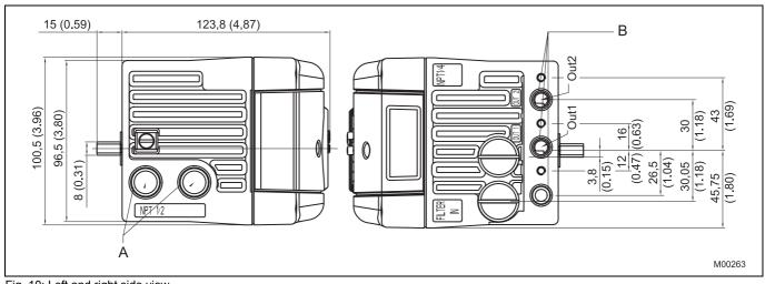
Fig. 10: Left and right side view
