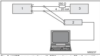
Fig. 6: HART communication with FSK modem via 20 mA signal line 3 Controller
