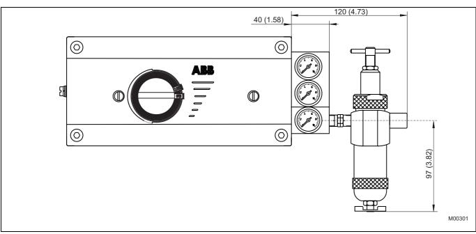
Fig. 13: Positioner TZIDC-200 with pressure gauge block and filter regulator
