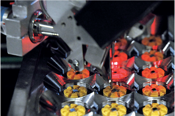
Fig. 11: Bonding of the silicon chip and the header
