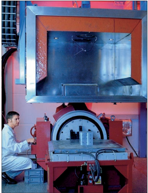
Fig. 19: Machine to perform the Highly Accelerated Life Test (HALT)
