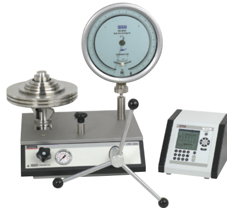
Pressure balance model CPB5000 with CalibratorUnit model CPU5000
