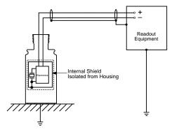
Figure 2: Multiconductor/Shield Configuration
