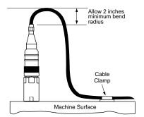
Figure 3: Cable Anchoring
