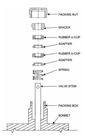
Figure 7 Rubber U-cup packing used for steam service. Packing Kit part number 81900-E1.
