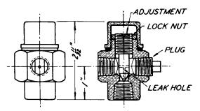
Most types of pressure regulators require a "feeler" pipe for best control. By using this adjustable orifice in the feeler pipe line, rapid pressure fluctuations will be dampened out and more steady control procured.
