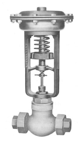
The setpoint is changed by varying the load on the adjusting spring. Rotating the ball-bearing adjustment wheel so as to compress the spring and increase its force against the diaphragm raises the setpoint. Rotation in the opposite direction lowers the setpoint. The scale along one side of the frame provides a reference for restoring the setpoint when adjustment wheel position has been changed from its normal setting.
