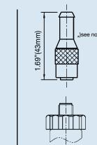
Flying leads conductor cross section up to max. 0.5 mm<sup>2</sup>/ AWG 20 with end splices, conductor outer diameter 6.8 mm, NEMA 4 / IP 67 Order code: DL
