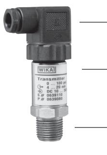
Standard electrical connection: DIN 43650 cap with solderless screw terminals. Available options include 1/2" NPT female conduit, NEMA 4 flying leads with vented cable, 4 and 6 pin Mil Plug, and custom connectors.
